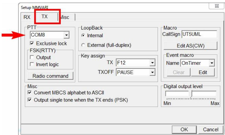
Select a serial port number which should be used for the PTT output (**COM8** in this example). Press OK to close this window.
