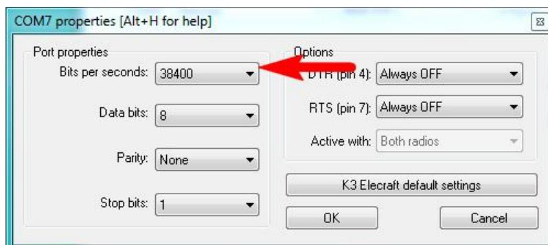
Select baudrate and the number of stop bits according to the user's manual of your transceiver. Click OK to continue.
