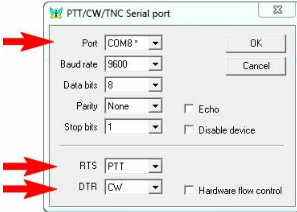
Select a serial port number which should be used for PTT and CW outputs (**COM8** in this example), and make sure RTS and DTR outputs are configured for PTT and CW, correspondingly. Press OK to continue.
