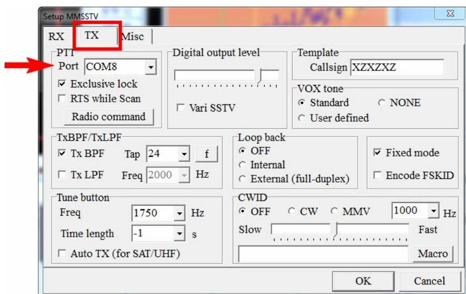
Select a serial port number which should be used for the PTT output (**COM8** in this example). Press OK to close this window.
