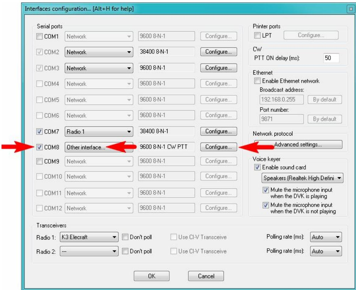
Check the box which corresponds to the PTT/CW port of the RigExpert WTI (**COM8** in this example). Select “Other interface” and then click “Configure”:
