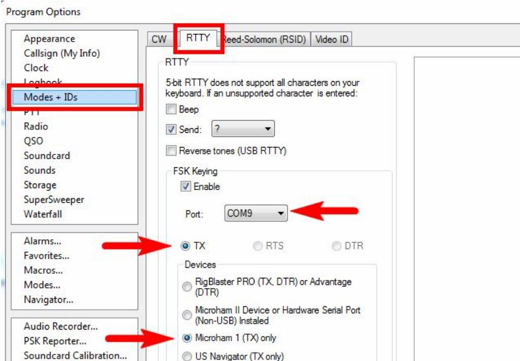
In the “FSK Keying” area, check the Enable box and select a serial port number which should be used for the FSK output (**COM9** in this example). In addition, select the “Microham 1 (TX) only” radio button.
