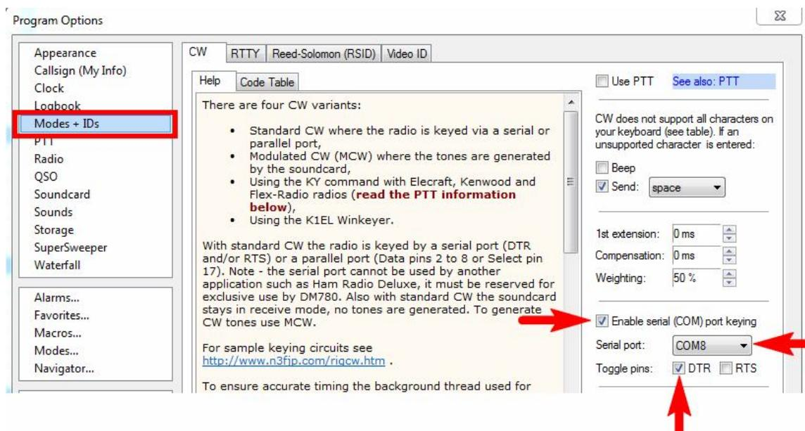
Check the “Enable serial (COM) port keying” and select a serial port number which should be used for the CW output (**COM8** in this example, same as the PTT port). Also check the “Toggle pins: DTR” box.
