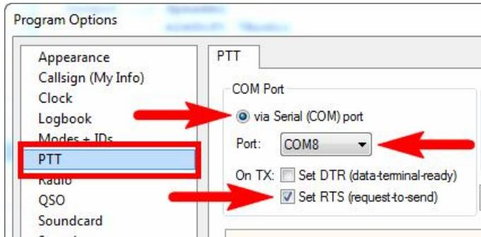
Select the “via Serial (COM) port” radio button, then select a serial port number which should be used for the PTT output (**COM8** in this example). Also check the “Set RTS (request to send)” box.
