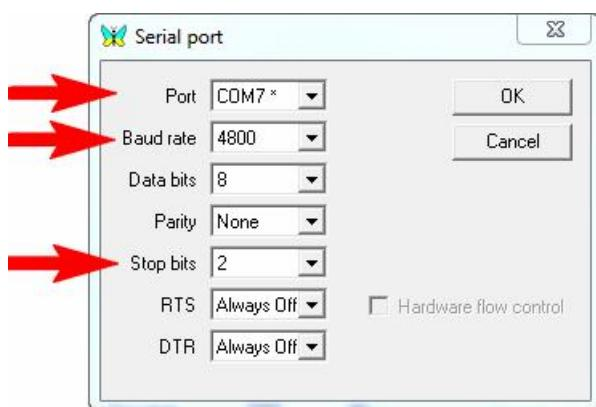
In the Serial port window, select a serial port number for the CAT system (**COM7** in this example). Select a baudrate and a number of stop bits according to the user's manual of your transceiver. Press OK to close this window, and then review other settings in the PTT&CAT dialog. Finally then press OK to finish.
