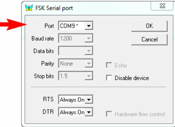
Select a serial port number which should be used for the FSK output (**COM9** in this example) and press OK to continue.
