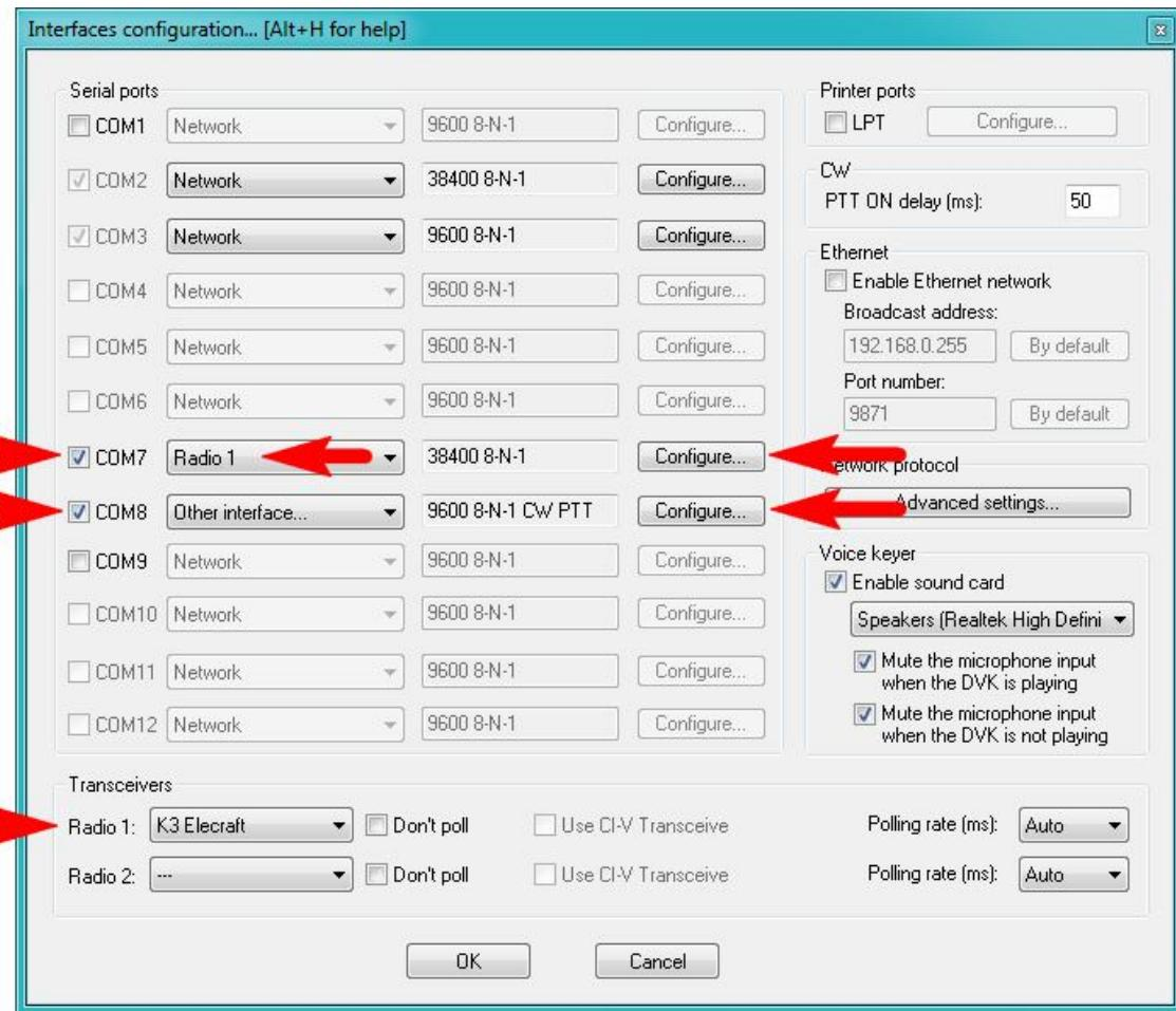
First, select your transceiver model (“Radio 1” at the bottom left of the window). Next, check the box which corresponds to the CAT port of the RigExpert WTI (**COM7** in this example). Select “Radio 1” and then click “Configure”:
