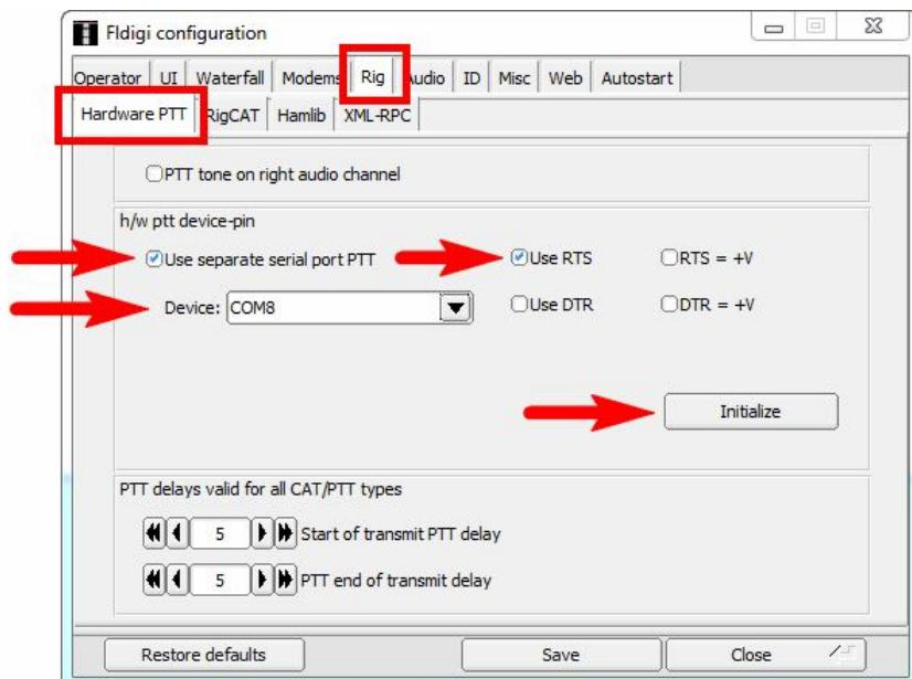
Check the “Use separate serial port PTT” and then select a serial port number which should be used for the PTT output (**COM8** in this example). Also check the “Use RTS” port box and press Initialize to open the serial port. Do not forget to press the Save button to save your settings.
