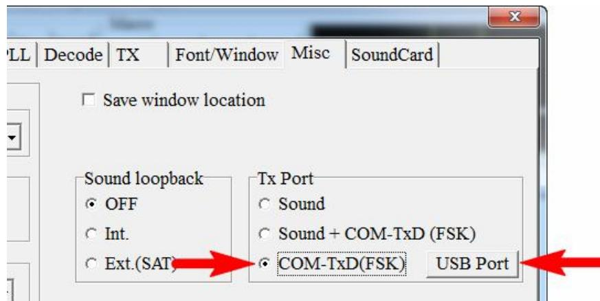
Select “COM-TxD(FSK)” in the “Tx Port” area and then press the “USB Port” button:
