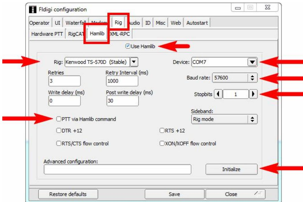
First, check the “Use Hamlib” box. Next, choose your transceiver model and uncheck the “PTT via Hamlib command” box. Select or enter a serial port number for the CAT system (**COM7** in this example). Select a baudrate and a number of stop bits according to the user’s manual of your transceiver. Finally, press Initialize to open the CAT serial port and then press the Save button to save your settings.
