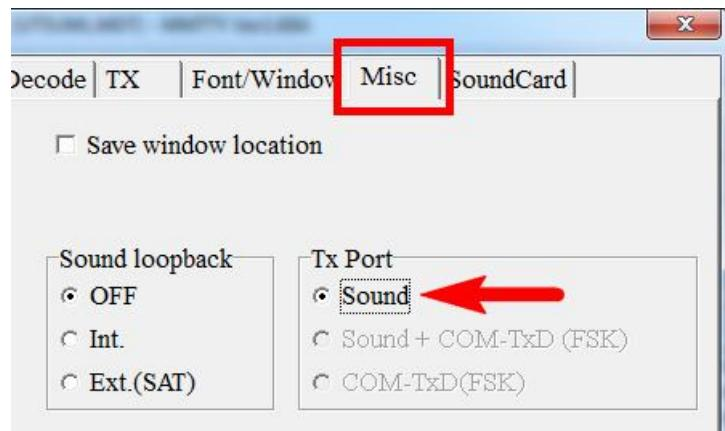
Finally, press OK in the “Setup MMTTY” dialog to apply new settings.
