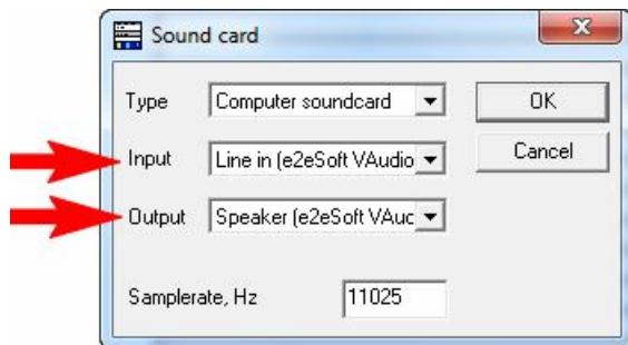
Select **e2eSoft VAUDIO** as both Input and Output and press OK to apply new settings.
