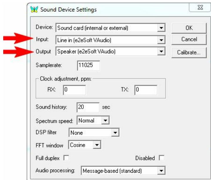
Select **e2eSoft VAudio** as both Input and Output, then check other settings and finally press OK to apply new settings.
