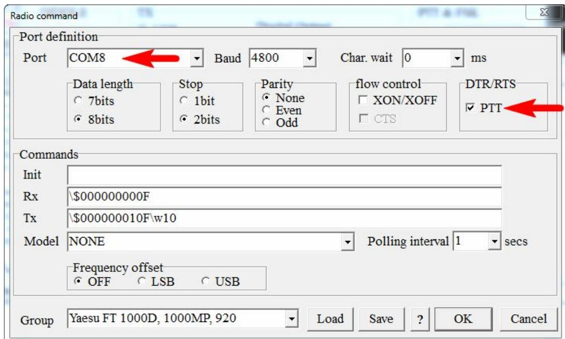
Select a serial port number which should be used for the PTT output (**COM8** in this example), and make sure the PTT box is checked. Leave all other settings unchanged. Press OK to close this window.
