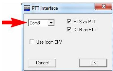
Select a serial port number which should be used for the PTT output (**COM8** in this example) and press OK to continue.
