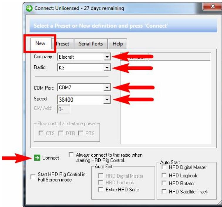
First, select your transceiver type and model. Next, select a serial port number for the CAT system (**COM7** in this example) as well as baudrate according to the user's manual of your transceiver. Finally, press Connect to let the HRD talk to your rig.
