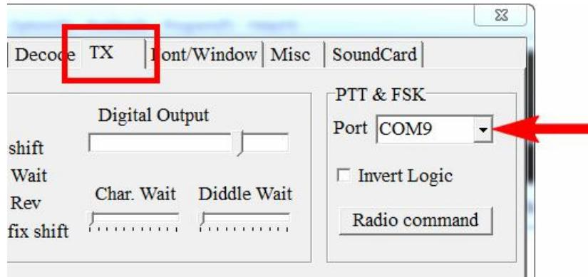
Select a serial port number which should be used for the FSK output (**COM9** in this example).
