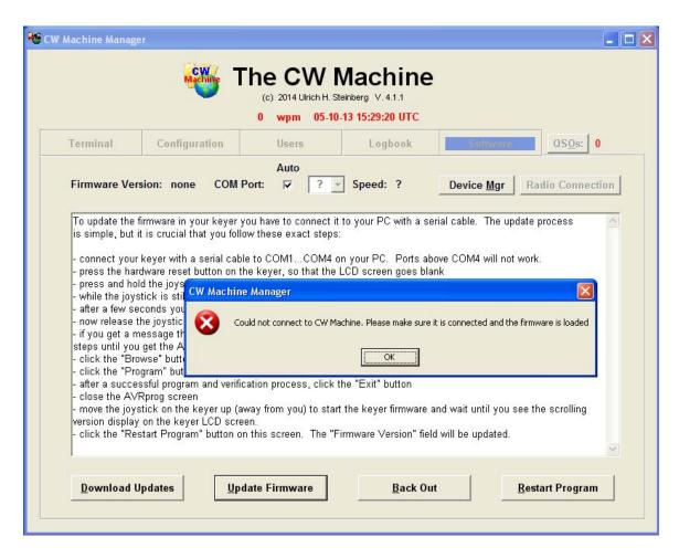
If you just forgot to connect the keyer, then all you need to do is to connect it and to click on the *Restart Program* button. After a successful connection the firmware version in the keyer and the connection port and speed are displayed at the top of the screen. The CW Machine Manager will scan all COM ports on your system to detect a CW Machine, unless you have unchecked the *Auto* box.
