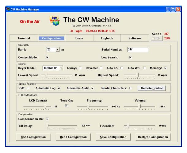
The **Keyer Speed** and the **UTC Time** are shown in the top section of the application window where they are visible on all screens. If you adjust the potentiometer on the CW Machine device, the speed change is automatically reflected on the screen. The UTC time is derived from your PC clock and the time zone that you have specified in Windows. When you start the CW Machine Manager, this time is sent to the keyer to synchronize its built-in clock which is
