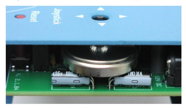
This knob cell can be used to keep the clock running for about a week in case of a power outage. You can also invoke all menu functions and even communicate via the serial port with only that knob cell. All other keyer functions, however, will not work when the device is powered only by this knob cell.
