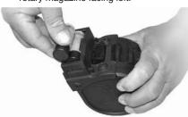
Once the selected magazine is loaded, insert the magazine into the bottom opening of the magazine well. The magazine should towards the rear of the shotgun (nearest to the receiver). The magazine should be until the locking latch is engaged. Verify the
