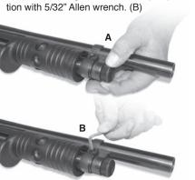
Reinstall shotgun stock; refer to the factory manual if necessary. **Note**: *If you have purchased a Venom-SE Kit, please refer to the M4 Stock Installation section.*
