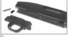
Remove the left and right side shell stop. **Note:** Only the left side shell stop will be installed during Venom Kit installation.
