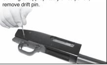
Remove the trigger group rear end first from the receiver. DO NOT PULL THE TRIGGER! Serious damage to the trigger group may result.
