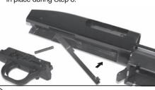
With safety on, install trigger group by first inserting front up into the receiver and then swinging rear of group up and into the receiver. DO NOT pull trigger during install.
