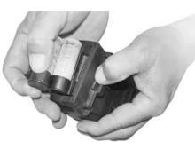
To clean the magazine, slightly depress the magazine shell follower and shake out or blow out loose debris. Wipe down magazine surfaces with plastic safe cleaners and lubricants.
