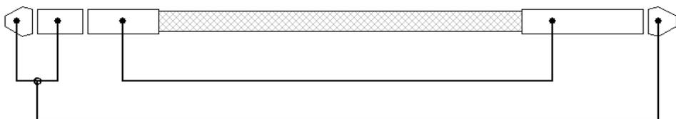
*Note: A stereo 1/8" patch cable with a stereo-to-mono adapter will not work!*
