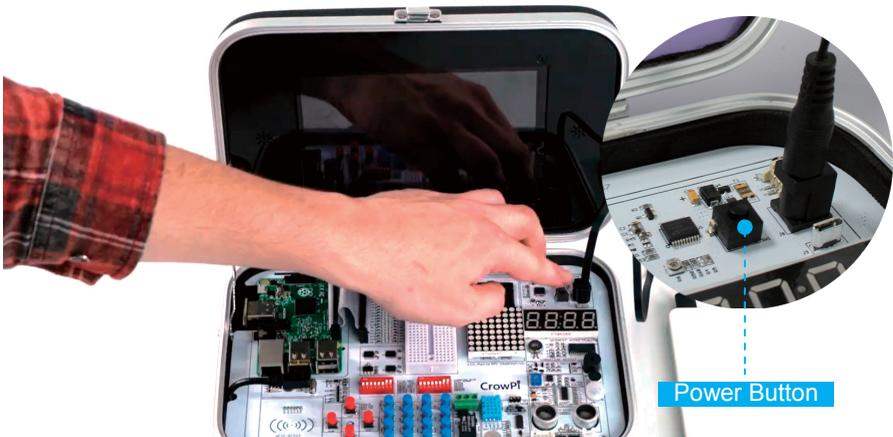
After powering on the board by clicking on the power button, the Raspberry Pi should load the operating system automatically. Give it few seconds up to one minute to load until you'll see the desktop environment and you'll be ready to go
