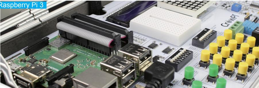
The second step will be plugging the “rainbow” cable into the CrowPi board. We'll take the other end of the “rainbow” cable and carefully plug it directly into the board making sure it covers all the pins and placed at the right spots.
