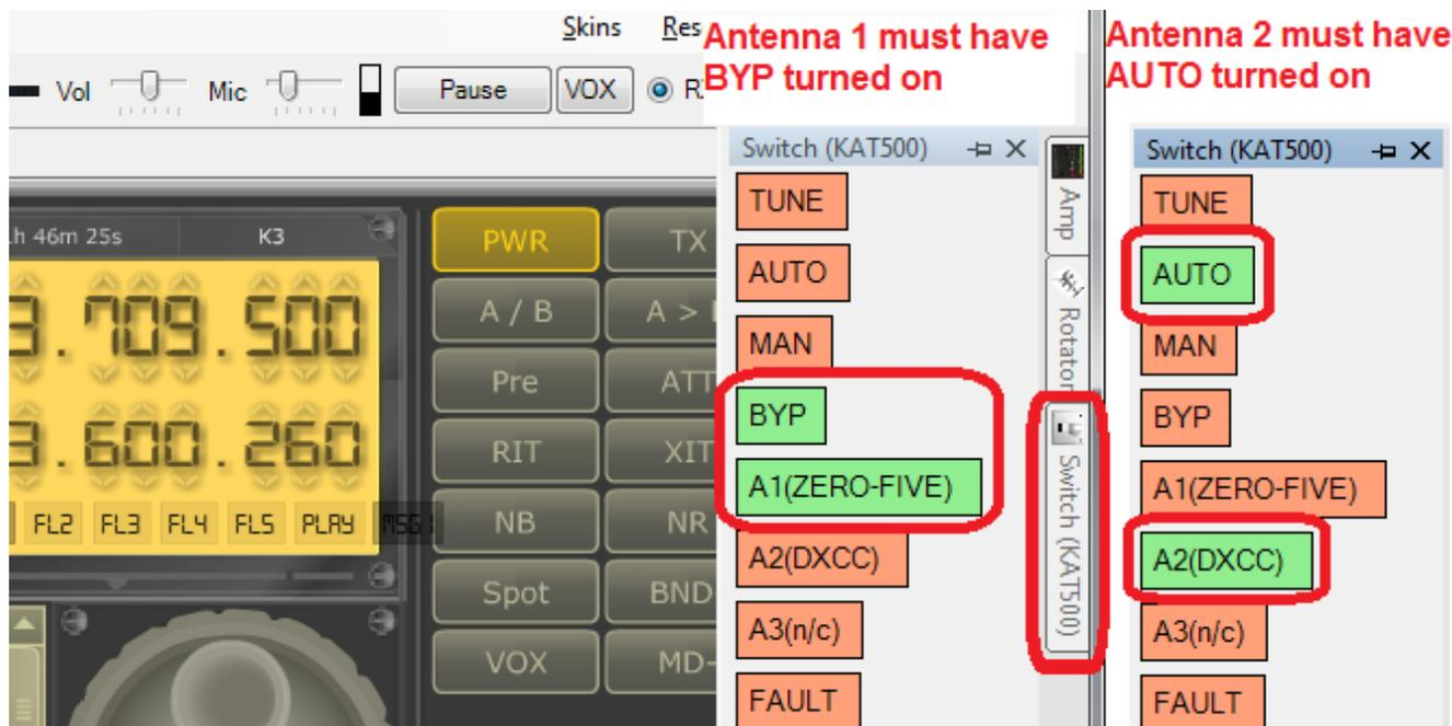
Either antenna is tuned by clicking the **M-Tune** button, which will cause the radio to transmit a low powered CW signal to force the appropriate tuner to tune the antenna for the new frequency. When the tuning cycle is complete, or 30 seconds has elapsed, the **M-Tune** button will turn off the tuning signal. When you click on **M-Tune**, wait for it to finish before clicking any other controls.
