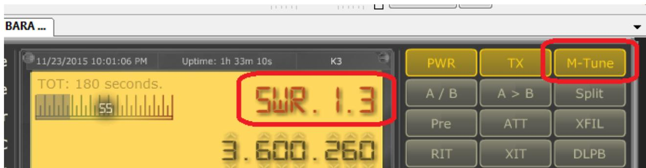
**If the SWR meter indicates a SWR greater than 2:1, do not transmit at that frequency.** Operating with a high SWR can damage the radio.
