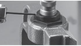
Once the die has been adjusted, tighten the setscrew to hold the proper setting
