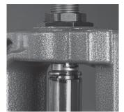
Place a bullet on top of the primed and powder-charged case.
