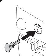
Push key into ignition slot. Be sure ignition key snaps into place.
