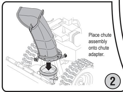
Shift Lever Upper Handle Handle Knobs Chute **Assembly Chute Control** Rod Chute Bracket **Chute Adapter**
