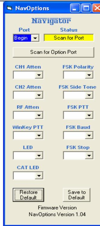
NavOptions scanned all possible COM ports looking for a Navigator Config port. It found Config on Port 12, and connected to it.
