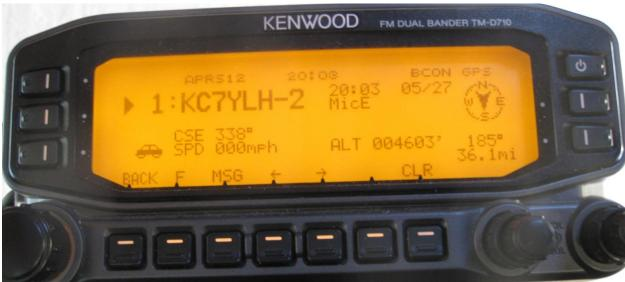
Use the arrow keys (bottom buttons, center) to move between the 3 APRS information displays. Page 1 isn't so helpful at first. Shown above is page 2 with the speed/direction of the target and the altitude (when reported). This is a very handy page for finding the HARBOR near-spacecraft! This tells you how far away and in what direction to look, it also tells you how high. (The ALTitude is referenced to sea
