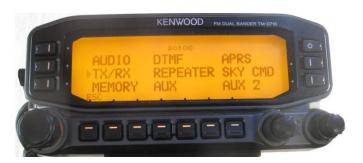
You can now rotate the channel select knob to move the pointer. Press the knob when the pointer is at APRS to access these settings. Be very careful here!
