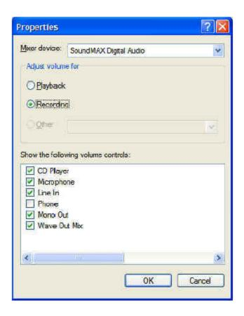
In Windows XP, make sure the Microphone slider is at mid-range and that there is a check in the Select box. If you are using a typical ham microphone, such as a Heil, and you have the "Advanced" button, click on it and select Mic Boost if that option is available, because it provides a 20-30 dB preamp. Now OK out.
