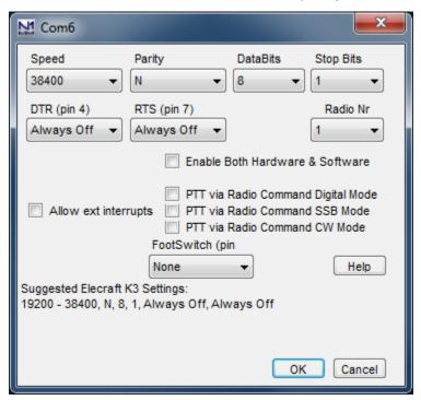
That will bring up this dialog, with connection details. Normally, N1MM Logger chooses the parameters in the first two rows for you, and does a good job. You might want to verify them with your radio manual, just in case. Radio/VFO number should be 1, so that your main VFO will be displayed in the main (first) entry window. The rest of the stuff on this dialog is not important right now, so just click OK to get back to the previous dialog, and then OK again to return to the Entry Window.
