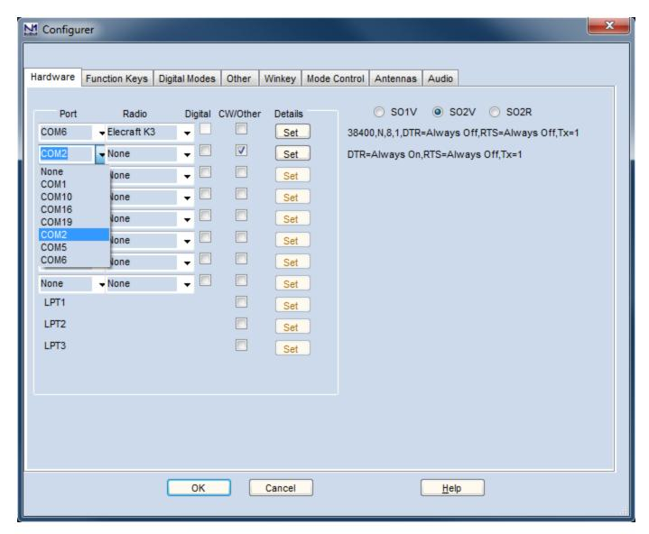
For this example, our CW port will be on the second port we configure (the first port, COM6, will be used for radio control). let's choose COM2 as our CW/PTT port. After selecting COM2 from the pull-down list of available ports, put a check in the CW/Other box and you'll notice that the Set button is no longer greyed. Click on it, and open the dialog for that port:
