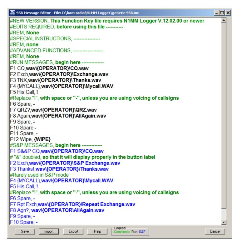
Don't be intimidated - we're just going to use this screen to set up a single function key to send a single message, so we can check out the entire flow from pressing a Function Key to having an audio message properly sent to your radio. The filenames and remarks you see in the editor now are the default filenames that are put into the table when you first install MM. If this is not your first time using N1MM Logger, these may not
