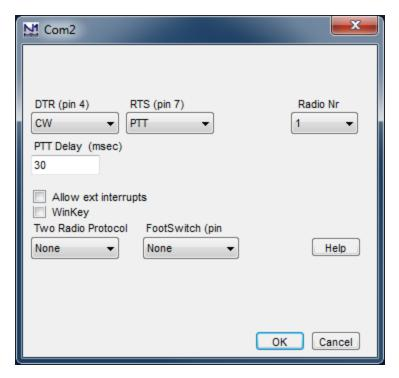
Set the Radio Nr to 1. The PTT Delay setting is to protect the relays in an amplifier by making sure that the T/R relay is closed before the program starts sending CW. The default value of 30 ms. is fine even if you don't have an amplifier.
