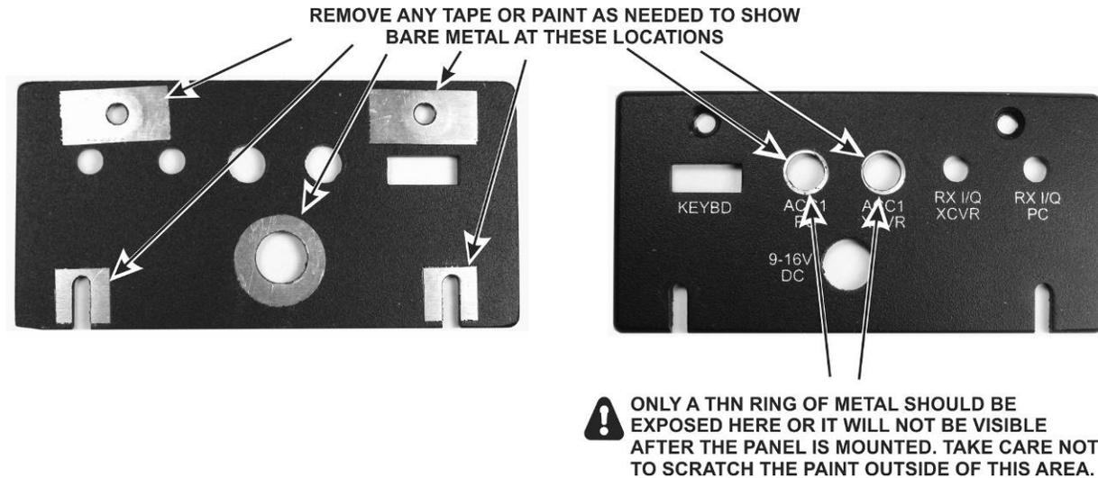
Figure 34. Preparing the Left Side Panel for Mounting.
