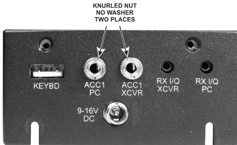
Figure 35. Mounting the Left Side Panel Part 1.
