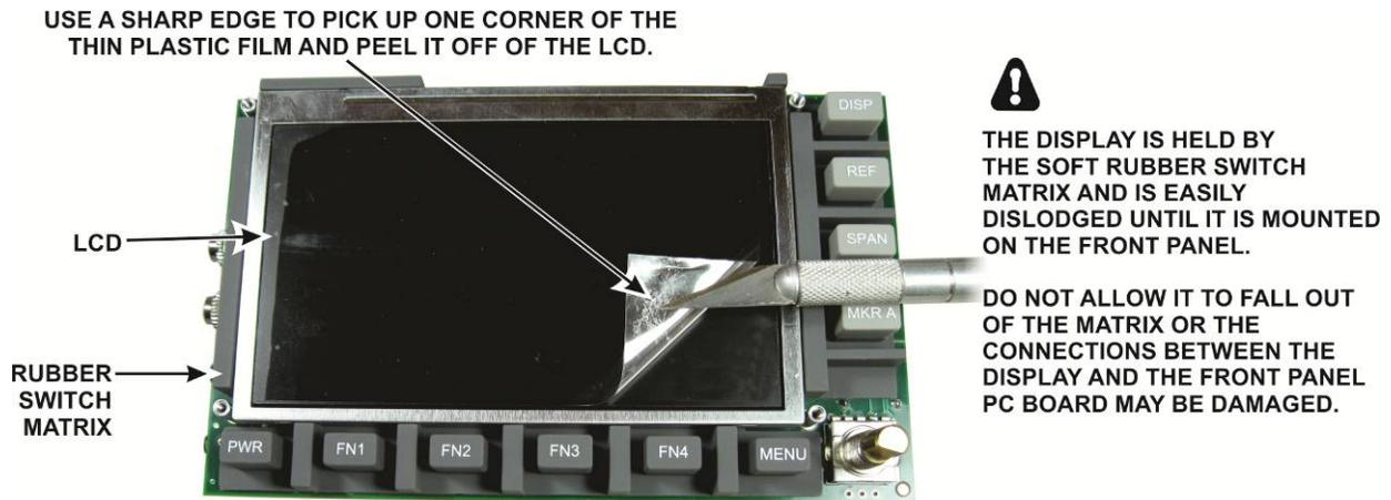
Figure 28. Removing the Plastic Film from the LCD.
