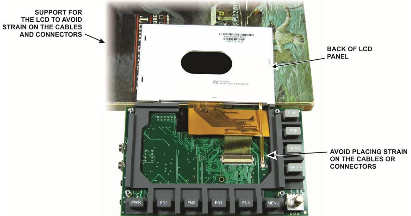
Figure 44. Removing LCD Panel from Rubber Key Matrix.
