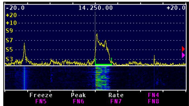
Figure 11. "U" Cursor on Upper Sideband Signal at 14.250 kHz.
