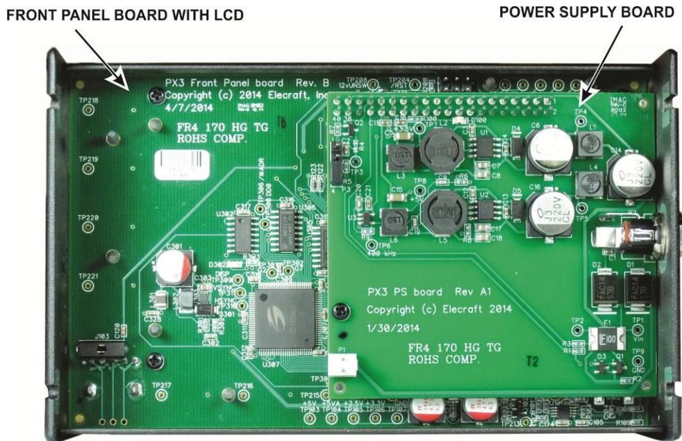
Figure 23 Assembled PX3 with Bottom Cover Removed.
