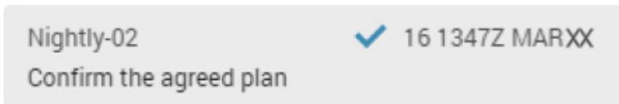
On the sender side, a returned receipt displays an additional checkmark along with a number saying how many of the recipients have sent receipts.
