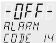
This excess temperature protection is independent of the control circuit. When activated heater and circulating pump are completely shut down. The alarm is indicated by optical and audible signals (continuous tone) and the error message "ALARM-CODE 14" appears on the VFD COMFORT-DISPLAY together with the ticker:
