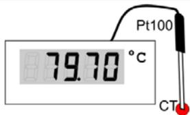
Read the value of measuring point CT on the device and enter under menu item >CALVAL X< by using the keypad.
