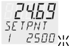
1. By pressing the key the circulator switches to the active SETPOINT< example on the left: >SETPNT / 1 25.00°C<. The integer digits flash (example: <25>).
