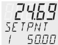
2. By pressing the keys and the value is changed to 50.00 °C and
