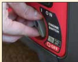
Fuel shutoff valve helps minimize stale fuel issues and makes storing easier.
