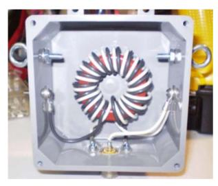
The AI4JU 4:1 current balun mounted in an electrical box (ccover removed)
