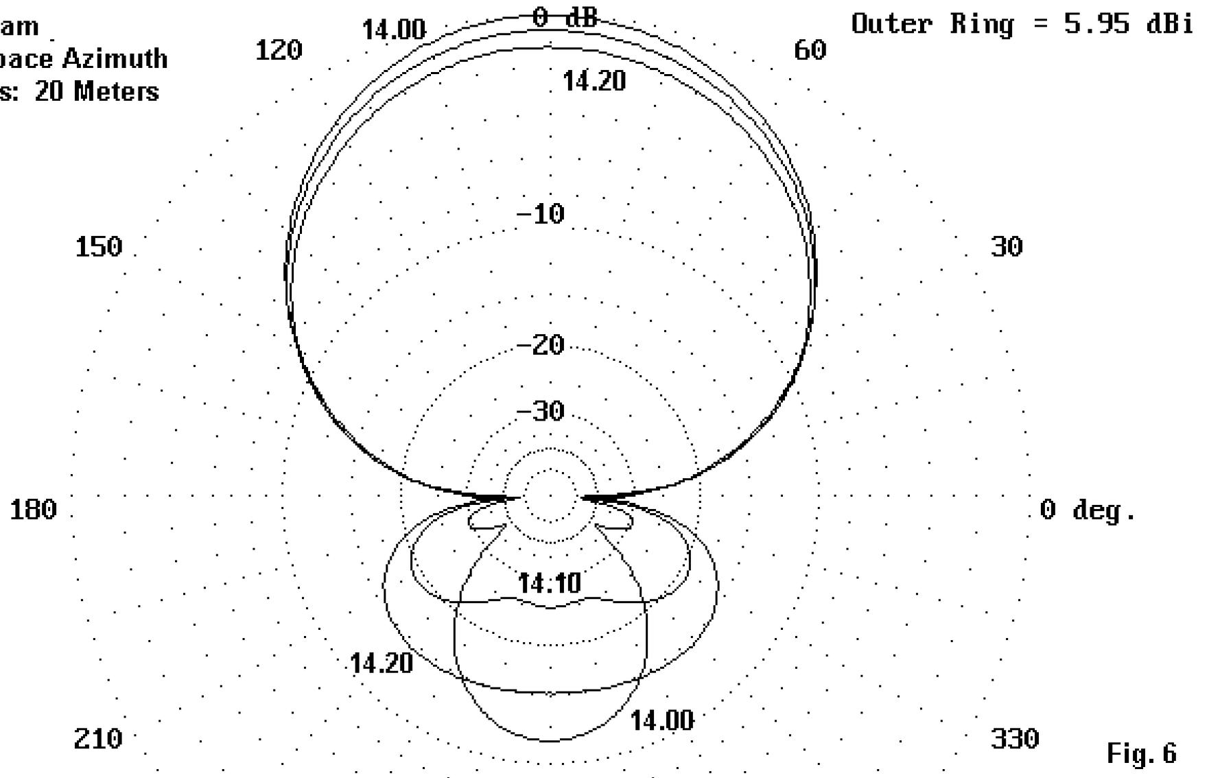
Hex Beam Azimuth Pattern
