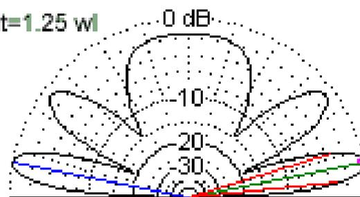
Elevation Patterns of a 29 MHz Dipole at Various Heights above Average Ground
