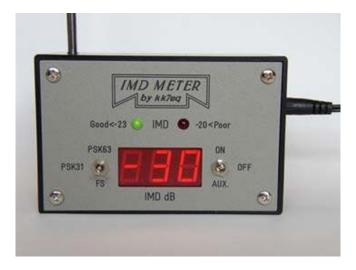
**Power Switch** - the right hand switch controls power to the meter. The center position is OFF, the up position selects the External +12.5 to +16 volt supply. The down position, marked Aux, is not used for normal operations, but may be used for short term battery operation of the meter. Battery connector is not supplied with the unit.
