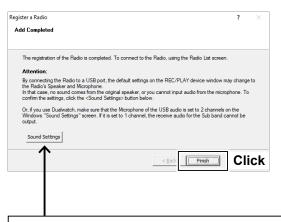
By connecting the transceiver to a USB port, the default settings on the REC/PLAY device window may change to the Radio's Speaker and Microphone. To confirm the settings, click <Sound Settings>.
