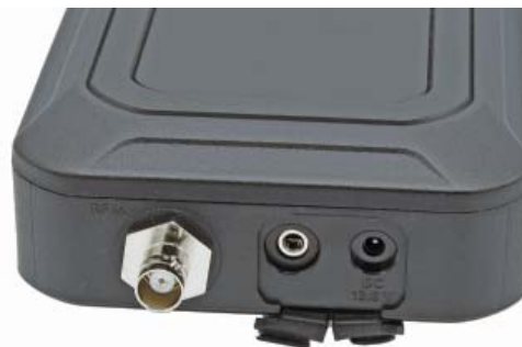
Figure 2 — One end of the Icom AH-705 has a BNC jack for RF from the transceiver, a jack for control signals from the transceiver, and an external dc power connector. The control and power jacks are protected by rubber covers when not in use.
