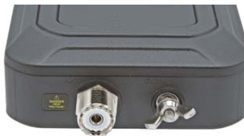
Figure 3 — The other end of the AH-705 has an SO-239 jack for the antenna feed line and a binding post for ground.
