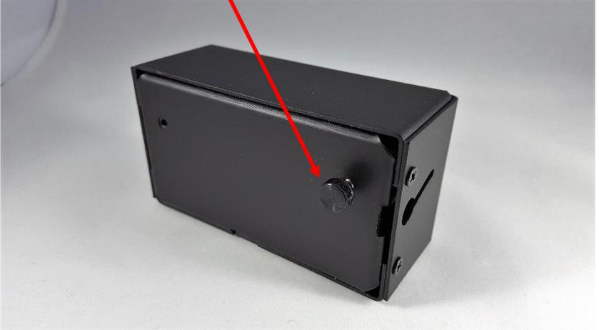
5. Install the KX3 mounting bracket under the thumbscrew as shown. Tighten the thumbscrew so the bracket is snug. The bracket edge should be even with the side of the SideKar.
