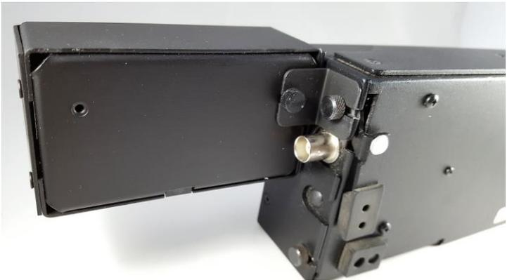
4. Lightly tighten the KX3 thumbscrew, and then swing the KX3 foot out to further tighten the foot. The SideKar should now be snug against the side of the KX3.
