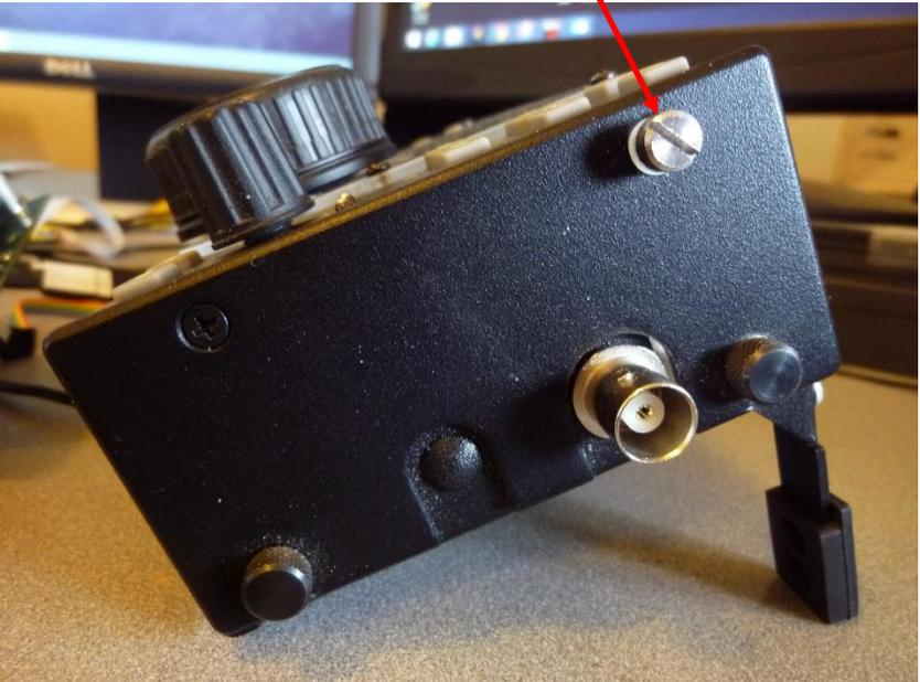
3. Loosen, but do not remove, the thumbscrew for the KX3 right foot. Fold the KX3 foot under the KX3 so it is not extended.
