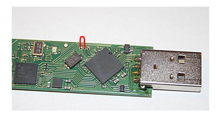
You need to connect the red marked points for example with tweezers **while** inserting the DV4mini into the USB interface. The boot loader will start with LEDs in color. Now you can start the user interface dv4mini. Go to expert settings load the new firmware by clicking on "Flash Firmware".
