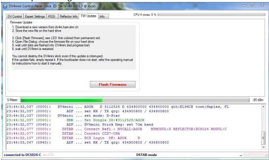
A file selection window opens and you select the new firmware file. This makes the LEDs on the DV4mini blink in different colors and when it is finished the blue light is on solid.
