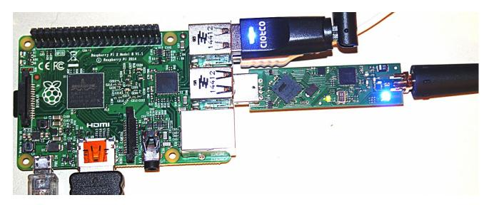
The dongle on the top is a WiFi stick to connect to the internet. Below you can see the DV4mini. The board also has connectors for a keyboard, a mouse and a HDMI display. This configuration allows for a low power operation.
