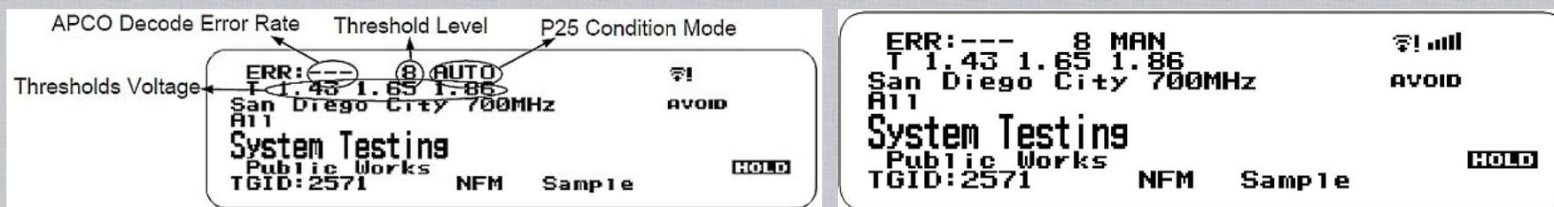
The first line on the display now shows the digital error rate and the decode threshold setting (0-20). The second line on the display shows the decode threshold levels.
