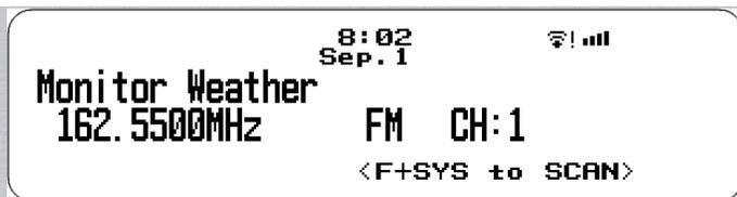
Press Channel to hold on any channel/frequency.
