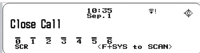
When the scanner detects a Close Call signal, CC Found! and Press Any Key appear for the length of time set in [Close Call Pause](#) or until the signal is lost.
