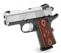
Caliber: 9mm Weight: 26 ounces Height: 5 inches Length: 6.5 inches Magazine Capacity: 9 Trigger: Long aluminum match-grade, 5 to 6 pounds Frame: Forged aluminum alloy. black hardcut anodized **Slide:** Forged stainless-steel. satin finish Recoil System: Dual spring, full-length guide rod Barrel: 3-inch stainless-steel match-grade, fully supported ramp **Grips:** Thinline cocobolo hardwood **Sights:** Fixed low-profile combat tritium 3-dot rear; dovetail front
