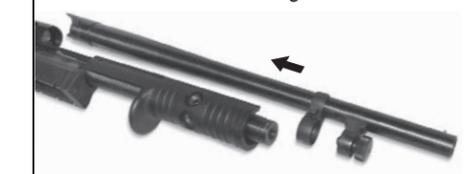
11 Tighten threaded capture nut into magazine tube (A). Tighten barrel clamp in position with 5/32" Allen wrench. (B)
