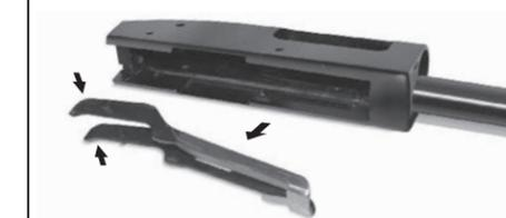
10 Use channel locks or pipe wrenches to remove factory magazine tube from receiver. **Note:** Removing the magazine tube will take a good amount of force to loosen the tube for unthreading. The use of a vise to secure the receiver will help with removing the magazine tube. Take caution not to scratch the receiver. Remove internal tube spring and follower plug. These components and the magazine tube will not be used for installation of the Venom Kit.
