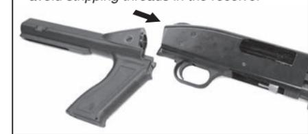
4 Remove mounting hardware (cast washer and bolt) from bag stored in rear stock tube. Assemble and insert mounting hardware into stock tube.
