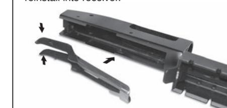
4 Reposition bolt back into shotgun receiver as shown.
