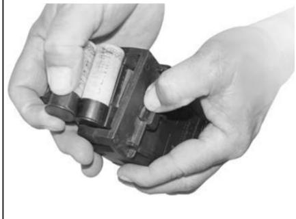
**5** To clean the magazine, slightly depress the magazine shell follower and shake out or blow out loose debris. Wipe down magazine surfaces with plastic safe cleaners and lubricants.
