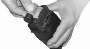
b. Rotary magazine; right hand shooters will load shells with the brass to the rear and the round portion of the rotary magazine facing right (as shown). Left hand shooters will load shells with the brass to the rear and the round portion of the rotary magazine facing left.
