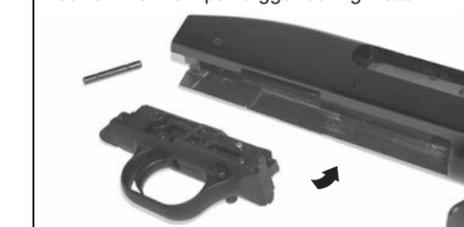
9 Reinstall drift pin through receiver to secure trigger group.
