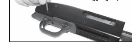
10 Partially open the breach by sliding the forend rearward. Reinstall barrel into receiver. Slide barrel clamp into position with open loop on barrel. Position barrel clamp just behind threaded barrel end. **Note:** Barrel clamp should not interfere with movement of forend during firearm use.
