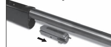
9 Remove shell lifter from receiver. Shell lifter is held in position by spring tension into corresponding holes in receiver. Squeeze ends to relieve tension for removal.
