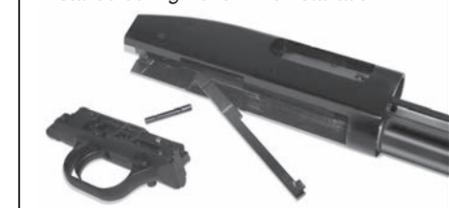
6 Position the bolt carrier as shown and remove it from the receiver.
