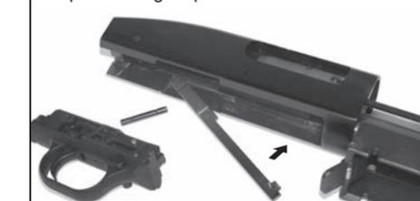
8 With safety on, install trigger group by first inserting front up into the receiver and then swinging rear of group up and into the receiver. **DO NOT** pull trigger during install.
