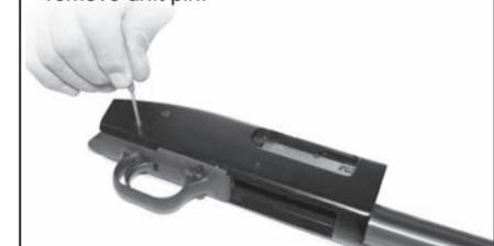
4 Remove the trigger group rear end first from the receiver. **DO NOT PULL THE TRIGGER!** Serious damage to the trigger group may result.
