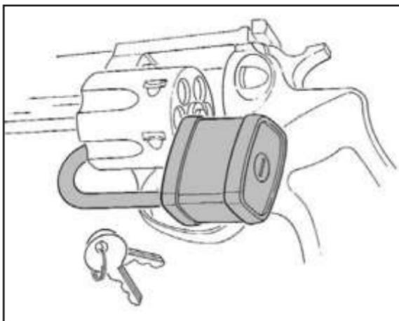
*Correct Installation of Lock
