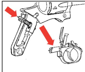
*NOTE: If you cannot supply sufficient force to the plunger using the mainspring assembly as a “tool,” then use a screwdriver of appropriate size and insert through hole in frame. It may be necessary to slightly depress the trigger while removing the trigger guard assembly.*
