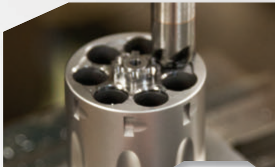
CHAMFERED CHARGE HOLES
