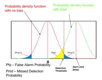
Figure 7. Integrity monitoring parameters.
