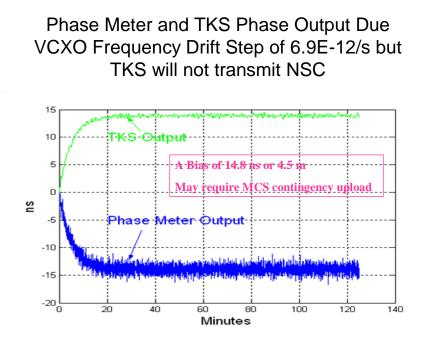
Figure 9. TKS phase transients due to a VCXO frequency drift jump.
