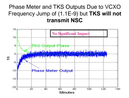
Figure 8. TKS phase transients due to a VCXO frequency jump.
