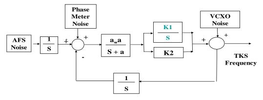
Figure 3 Simplified TKS Error Model in S Domain
