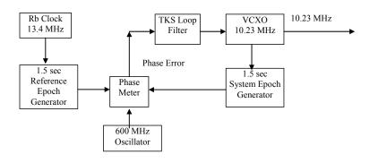
Figure 1. Simplified TKS block diagram.
