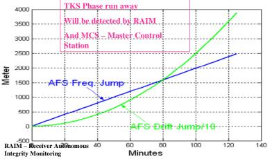
Figure 10. TKS phase runaway due to a RAFS frequency jump and frequency drift jump.
