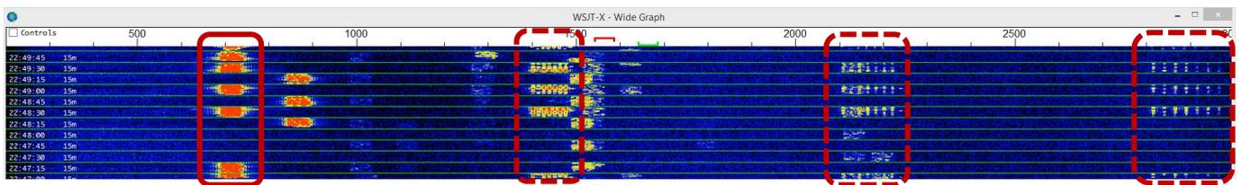
4.3 Setting your transmit levels is a bit more complicated than it seems: **simply adjusting the rig’s power output control is not sufficient** as even QRP signals can be rotten if the audio circuits are overloaded.
