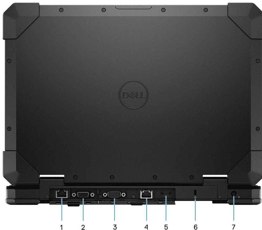
1. Ethernet Port (Optional Rear configurable I/O)
