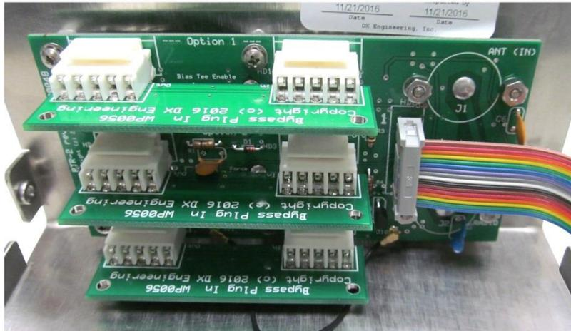
To remove the Bypass Plug-In board, use a small diameter Phillips Screw Driver. Put the screw driver through the hole on the corner of the board to be removed and gently pry it slightly outward. Move the screw driver to the other corner of the board to be removed and repeat the prying action. The board will come loose from the board connectors and be able to be easily removed. Repeat the same sequence for the other Bypass Plug-In boards See the photos below.
