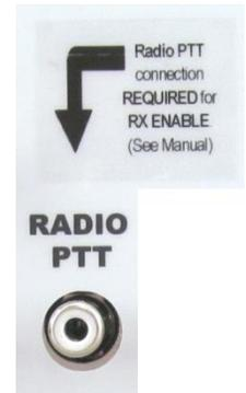
When we turn the RTR-2 on, we still want the same connections, the **RADIO** to **MAIN ANT IN**, when the transceiver is keyed to transmit, or when we want to listen only to the transmit antenna (**MAIN ANT**). Okay, let's tell the RTR-2 when it is safe to switch to receive mode. Well, unfortunately, we can't because transceivers don't put out an "Okay to Receive" signal, they only send out a "Hey, I'm transmitting signal" on the amplifier keying line (which we connect to **RADIO PTT**).
