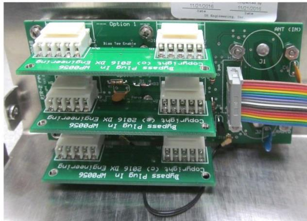
Remove the Option 1 and Option 2 By-Pass Plug In boards to have a clear view and easily check/change the jumpers. Refer to “*Removing Bypass Plug-in Boards*” for removal or installation of these boards.
