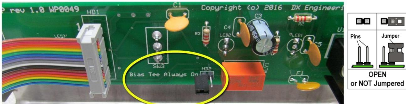
When this jumper is connected (both pins shorted together), bias tee voltage is present regardless of transmit and receive keying. This jumper should only be installed for non-RTR, receive only use of the RTR-2. Keyed bias tee voltage on the receive feedlines is normally desired.
