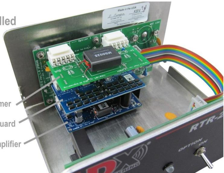
Note: Because of the power and switching requirements, the Receive Preampifier **DXE-RPA-2-PM** must be installed in only the Bottom position. When installing an optional module or a Bypass board, ensure the pins are properly aligned and push the board fully in place.
