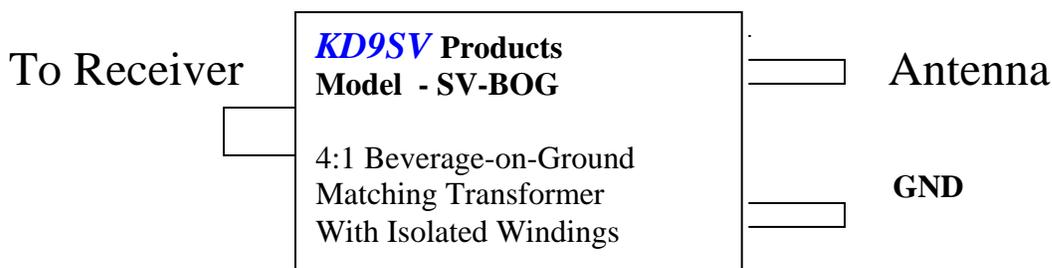
This Transformer will match the 200 ohm Beverage Antenna impedance to the 50 ohm impedance of your Coax resulting in the proper transfer of signals to your receiver.
