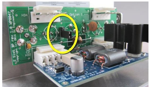
Alternatively, if the RPA-2 is to be located at the receive antenna, the unit may be powered from DC on the feedline that is connected to the “**RECEIVER OUTPUT**” connectors. This requires a user supplied bias-tee or feedline voltage inserter used at the operating position, providing the properly filtered and regulated (center-positive) +13.8 Vdc, 140 mA minimum.
