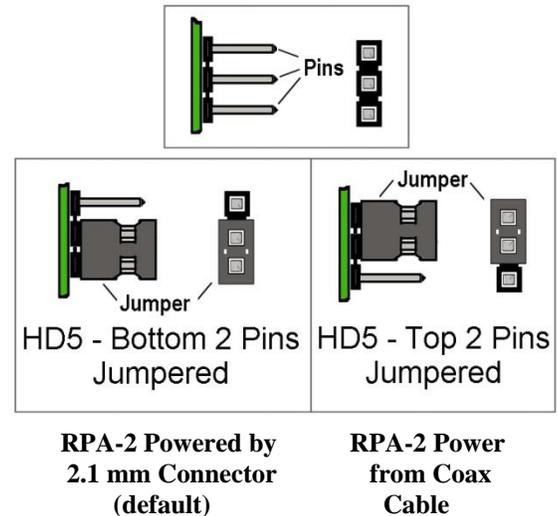
**NOTE:** The ability of the RPA-2 to be powered on the “**RECEIVE OUTPUT**” coaxial cable cannot be extended to the antenna feedline. In other words, when the RPA-2 is powered on the coax, any active devices used on the “**ANTENNA INPUT**” side of the preamplifier will require separate power connections.
