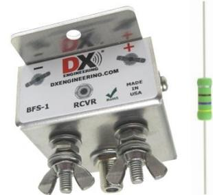
The feedline impedance of the **DXE-BFS-1** is optimized for 75  $\Omega$ , however, any feedline between 30  $\Omega$  and 100  $\Omega$  can be used. While not intended for transmitting, the **DXE-BFS-1** can withstand power levels of 20 watts continuously, 200 watts for 5 seconds or the power rating of the termination resistor, whichever is less. The **DXE-BFS-1** coaxial cable connection uses an industry standard CATV F type connector.
