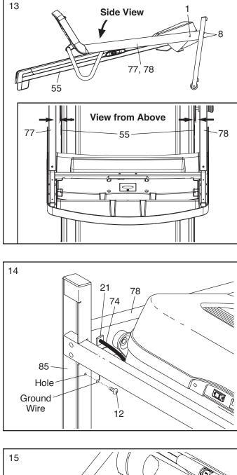
14. Attach the ground wire on the Upright Wire (74) to the indicated hole in the Base (85) with a #8 x 1/2" Screw (12).
