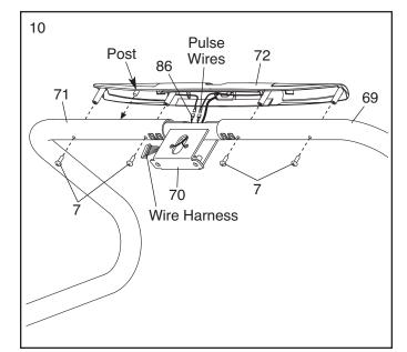
11. Hold the handrail assembly near the console assembly. Connect the wire harness extending from the handrail assembly to the wire harness extending from the console assembly. See the inset drawing in step 7. The connectors should slide together easily and snap into place. If they do not, turn one connector and try again. IF YOU DO NOT CONNECT THE CONNECTORS PROPERLY, THE CONSOLE MAY BECOME DAMAGED WHEN YOU TURN ON THE POWER.
