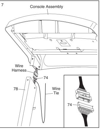
8. Insert the wires into the Right Upright (78). Next, insert the brackets on the console assembly into the Right Upright and the Left Upright (77). **Be** careful not to pinch any wires.
