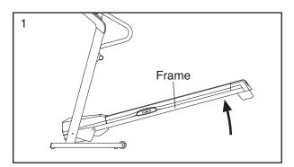
2. Hold the treadmill firmly with your right hand as shown. Pull the latch knob to the left and hold it. Raise the frame until the hole in the platform cushion is aligned with the latch pin. Then, slowly release the latch knob; **make sure that the latch pin is fully inserted into the platform cushion.**
