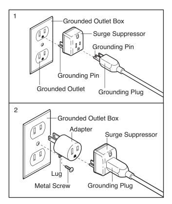
The temporary adapter should be used only until a properly grounded outlet (see drawing 1) can be installed by a qualified electrician.
