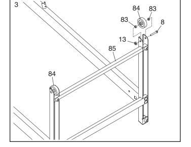
4. Raise the Uprights (77, 78), and position the Base (85) near the treadmill as shown.
