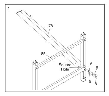
Orient the Left Upright (77) as shown, and attach it to the Base (85) with two 3/8" x 2 1/4" Bolts (8) and two 3/8" Star Washers (9); do not tighten the Bolts yet.
